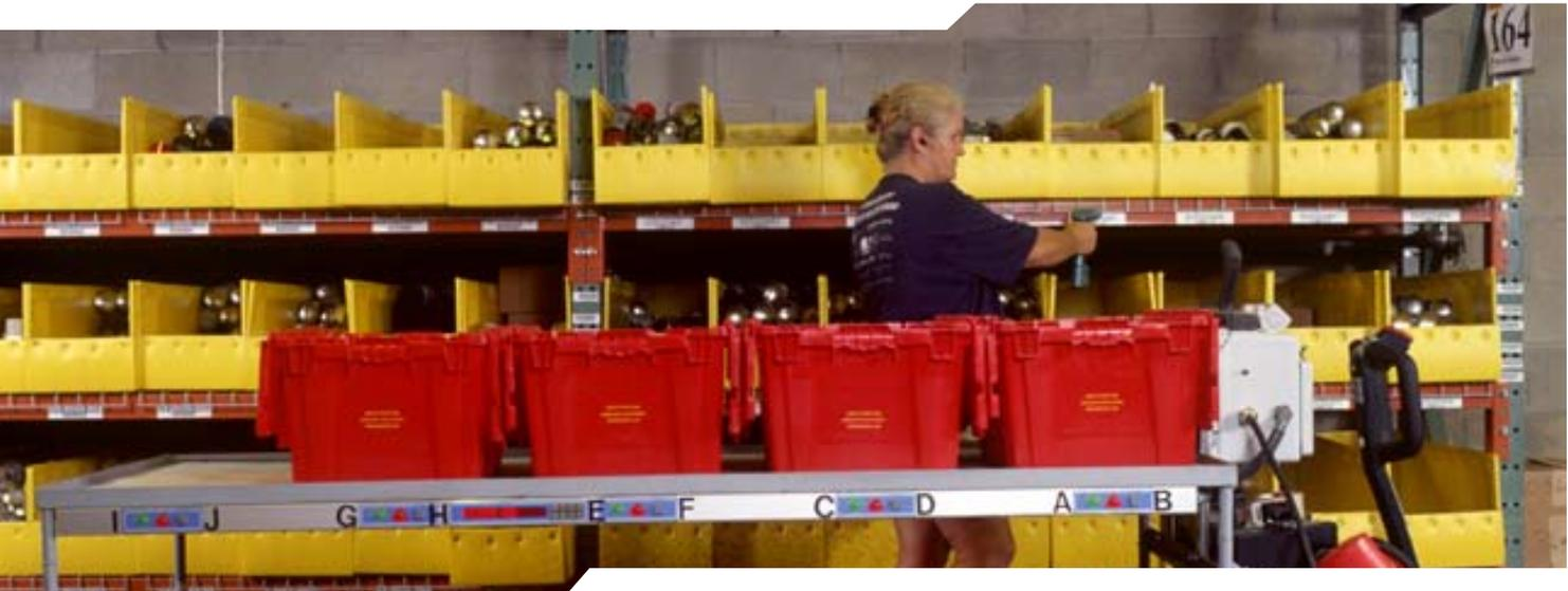
conveyors in the pick-to-light areas increases ergonomic safety by reducing heavy lifting and also eliminates wasted movement, thereby speeding up the picking process.
